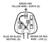
The BLUE wire must be connected to the terminal marked with the letter N
