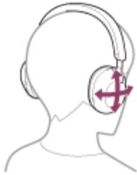
If you put on the headset without adjusting the slider, the headset may not be positioned properly on your head, resulting in discomfort or a weak noise canceling effect. The wearing detection function of the headset may also not work properly and cause music playback to stop automatically or activate the automatic power off function (the battery saving function) to automatically turn off the headset.
