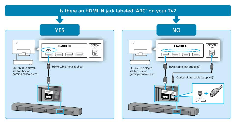
\* If your TV does not support the ARC (Audio Return Channel) function, connect an optical digital cable (supplied) to listen to the TV sound.
