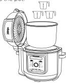
2 Assemble the pressure lid by aligning the arrow on the front of the lid with the arrow on the front of the cooker base. Then turn the lid clockwise until it locks into place.
