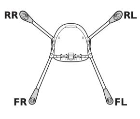
4. Slot the end of the footrest into the housing on the underside of the seat. Push the leg rest in until it locks into the housing.
