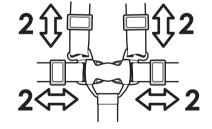
9. To open the harness, push the locking tabs inwards (1) and slide the two waist strap tabs out of the buckle (2).
