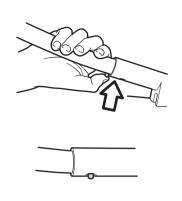
3. Slot the feet onto the ends of the legs. Ensure the feet are slotted onto the correct legs. The base of the feet are marked with two letters, see diagram for the correct fitting.
