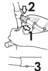
2. Slot the two back legs into the rear housing on the seat. Push the pins on the legs inwards and fully insert into the housing. Ensure the pins are protruding through the holes in the housings after fitting.
