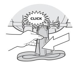
5. Attach the tray support to the front of the seat. Slot the tabs on the back of the support into slots in the seat (1). Rotate the support down until the front locks onto the seat (2).
