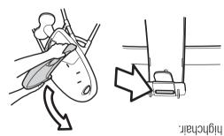
rotate the support upwards until it comes free of 11. Turn the locking button anti-clockwise and
