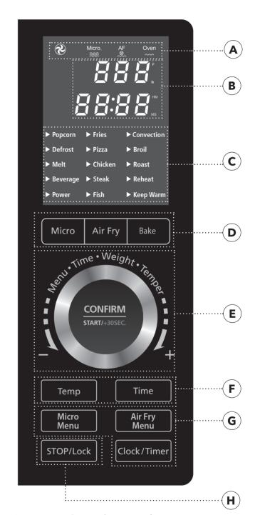
**STANDBY MODE:** When no cooking program is running, the appliance is in standby mode. In standby mode, only the time is displayed; the other icons are not illuminated.
