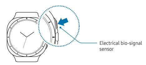
The measurement will start and the ECG wave will appear on the screen.
