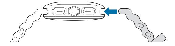
2 Gently pull on both sides of the band to make sure it is tightly connected and not detached from your Watch.
