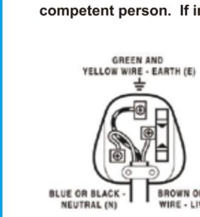
The BLUE wire must be connected to the terminal marked with the letter N. The BROWN wire must be connected to the terminal marked with the letter L. The GREEN & YELLOW wire must be connected to the terminal marked with the letter E or the earth symbol .
