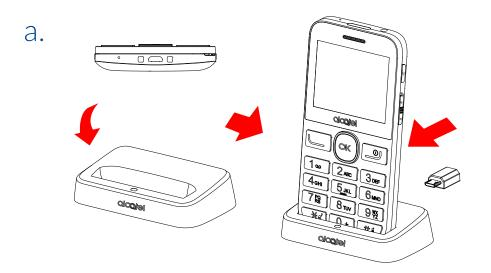
To charge the phone, you can place the cradle charging connector of the phone to the cradle, then connect battery charger to the cradle and plug into the socket.
