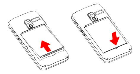
Unclip the cover, then remove the battery.
