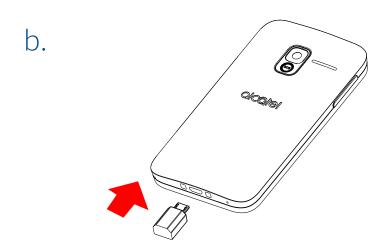
Connect battery charger to your phone and plug into the socket
