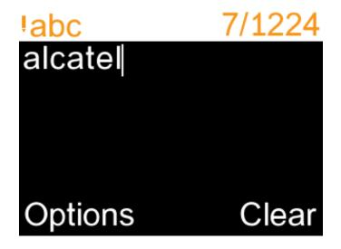
To insert a punctuation mark or special character, press 0+ key.
