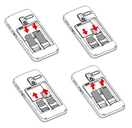
Place the SIM card with the chip facing downwards and slide it into its housing. Make sure that it is correctly inserted. To remove the card, press and slide it out.
