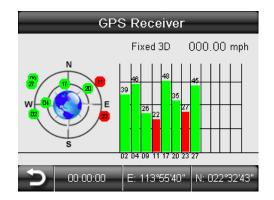
This page gives your current position in degrees longitude and latitude, your current speed and the status of your position, i.e. Fixed 3D or Fixed Invalid etc. The compass circle shows the satellites that the unit is receiving and the bar chart shows the signal strength for these satellites
