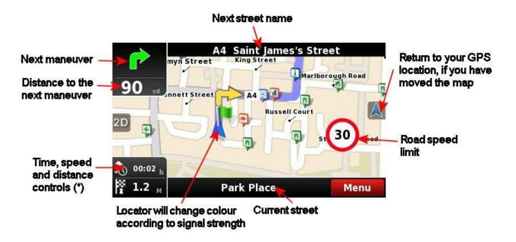
(\*) – Time, speed and distance controls show different information. Tap each in turn to toggle between the alternative modes as shown below.
