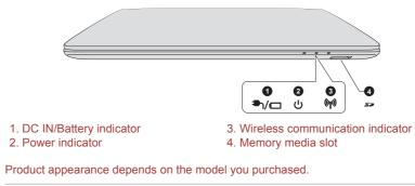
■ ✓ ■ DC IN/Battery indicator The DC IN/Battery indicator shows the condition of the DC IN and the battery's charge - white indicates the battery is fully charged while the power is being correctly supplied from the AC power adaptor. Please refer to the *Power Condition Descriptions* section for more information on this feature.
