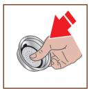
Dry with a cloth. Put the perforated filter back in the housing and press as far as it will go
