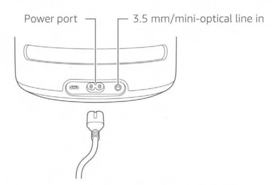
To connect an audio component such as a CD player or MP3 player, use the combination 3.5 mm/mini-optical line in on the back of your Echo Studio.
