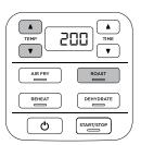
**NOTE:** It is recommended to let the unit preheat for 3 minutes before adding ingredients. If preheating, skip step 4, insert the empty pan and press the START/STOP button to begin.
