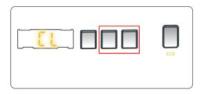
If any button is pressed or the selected programme is changed by the programme dial while the child lock is active, the "CL" symbol will flash on the electronic display for 2 seconds.
