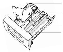
Liquid Detergent Apparatus Main wash detergent compartment Softener Compartment Pre-wash detergent compartment
