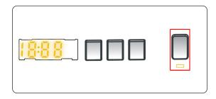
By pressing on the Start/Pause button, you may start the programme you have selected or suspend a running programme. If you switch your machine to the standby mode, the Start/Pause led on the electronic display will blinkdisplay will blink
