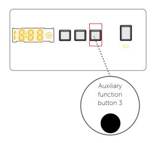
You can use this auxiliary function to delay the start time of the washing cycle for 1 to 23 hours .
