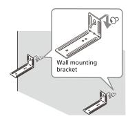
8 Put the bar speaker on the wall mounting brackets.
