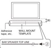
5 Fasten the screws prepared in step 1 securely into the screw marks on the "←③ SCREW LINE" printed on the WALL MOUNT TEMPLATE.
