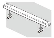
9 Align the positions of the screw holes on the bottom of the bar speaker and holes of the wall mounting bracket, then fix the bar speaker to the wall mounting brackets by fastening the screws (supplied) securely.
