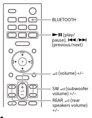
Press and hold the BLUETOOTH button for 2 seconds.
