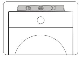
**2.** Level the washing machine by manually adjusting the levelling feet.
