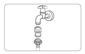
Before connecting the water hose to a water tap, connect the supplied check valve to the water tap and then connect the water hose.
