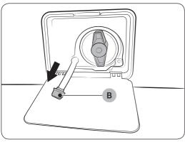
**3.** Place an empty, spacious container around the cover, and stretch the emergency drain tube to the container while holding the **tube cap (B)**.
