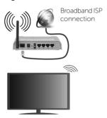
A Wireless-N router (IEEE 802.11a/b/g/n) with simultaneous 2.4 and 5 GHz bands is designed to increase bandwidth. These are optimized for smoother and faster HD video streaming, file transfers and wireless gaming.
